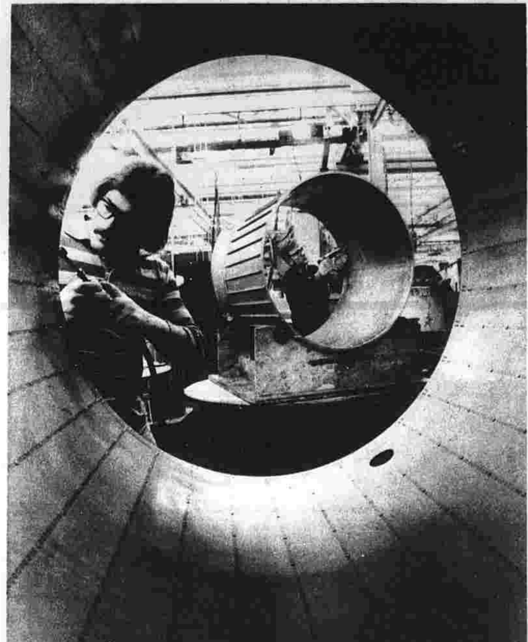
Employees of Pratt and Whitney Aircraft in East Hartford do some delicate work here on the augmentor case from an F100 engine. The F100 powers the F-15 and F-16 fighters.
